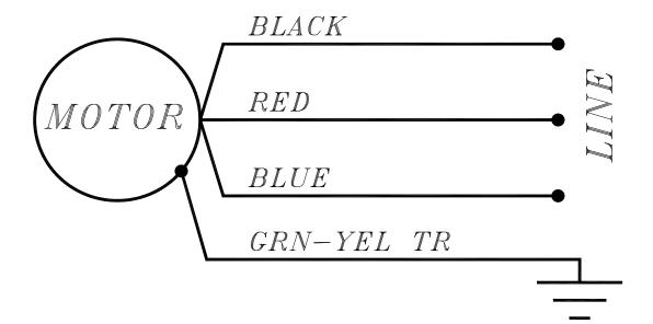
TO REVERSE DIRECTION OF ROTATION, TRANSPOSE ANY TWO LINE LEADS.
